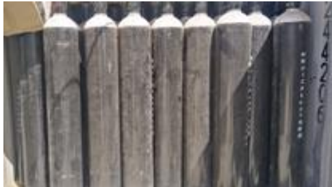
Oxygen cylinders were dumped in a container without temperature & humidity measures since 2019-20
